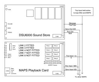
components must be fitted and all Ext clock links must be cut. Sync links must be cut on all slave boards.
